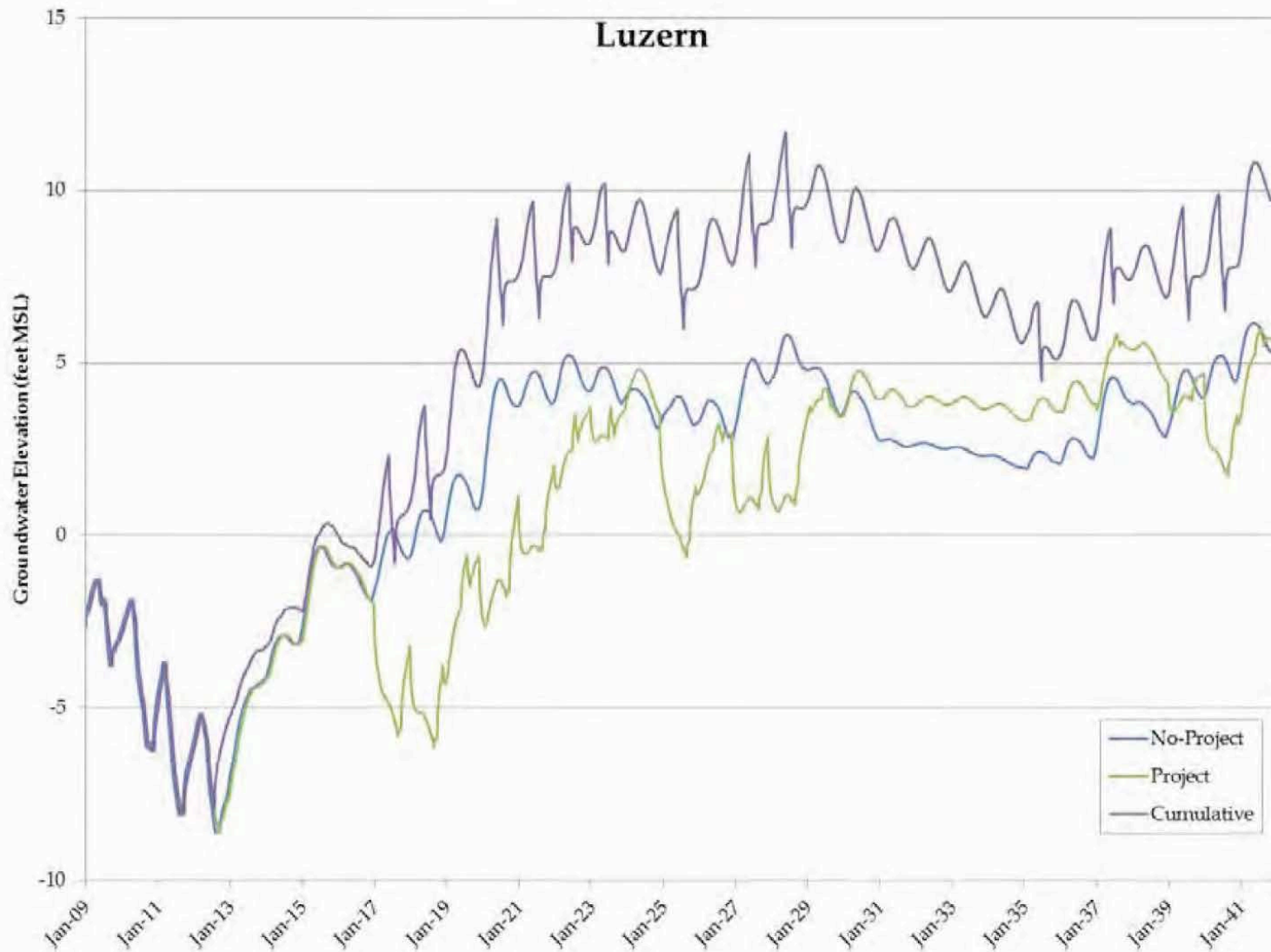
Figure 16: Predicted Static Groundwater Elevations at Luzern Well
